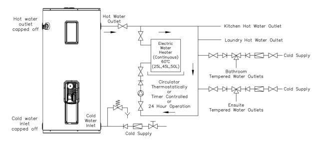
Circulated Hot Water Flow and Return System Grid Interactive or PV Powered Electric Water Heater
